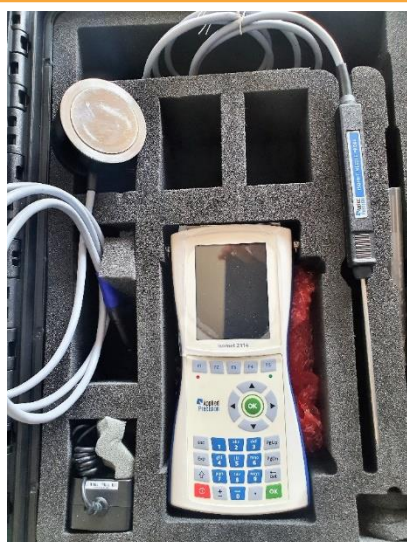
Figure 1. The ISOMET 2114 thermal conductivity measurement system
