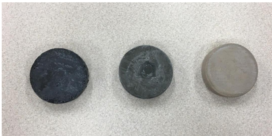
Figure 2. Hardened cement slurries in the form of discs.
