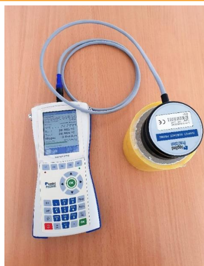
Figure 2. Measurement of thermal conductivity of a cement sheath sample
